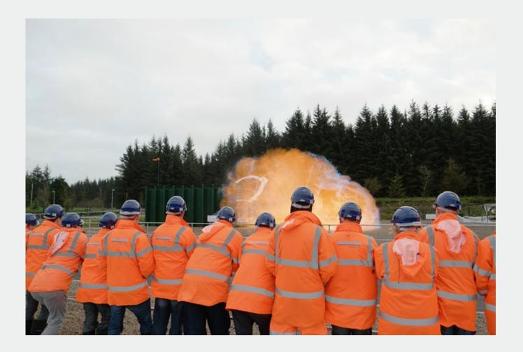
An 80 m<sup>3</sup> chamber is filled with stoichiometric propane/air mixture. The gas mixture is ignited resulting in an explosion allowing the delegates to experience a 25 mbar pressure wave.
