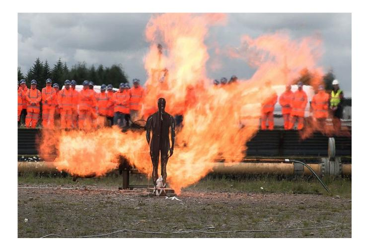
Natural gas release through a valve spindle packing area. The released gas is ignited immediately and the pressure is gradually increased to 15 bar.
