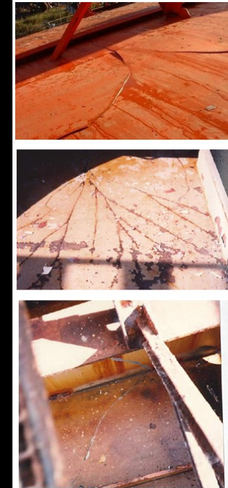
Roue (2011)- Steel fractures on actual LNG assets due to cryogenic spills
