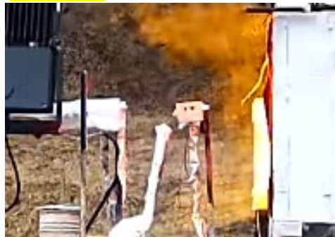
Test 6 - full tank blowdown from a tank pressure of 896 bar, after 4 minutes (at 250 bar)
