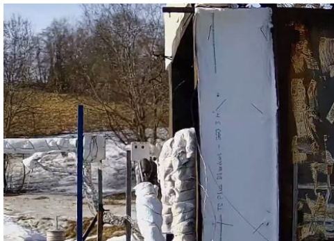
Test 1 - constant pressure release at 250 bar
