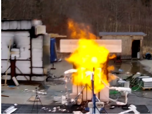
Test 6 - full tank blowdown from a tank pressure of 896 bar, start of test
