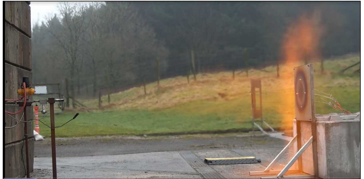
Jet blowdown, 350bar, 3.3m standoff distance, 5mm nozzle. Still of visible recording (5 secs approx. into release)
