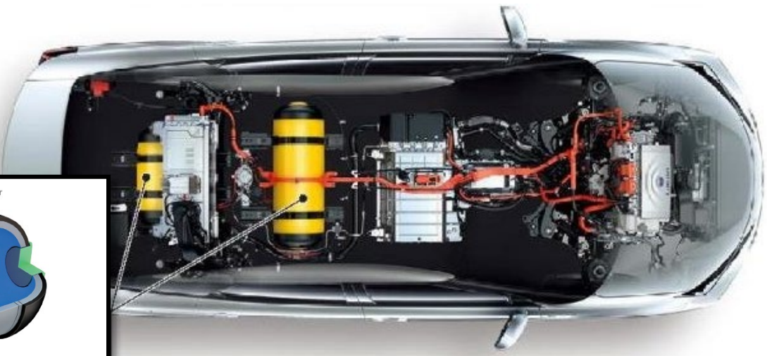
Toyota Mirai hydrogen fuel tank ( www.car.nulisen.com )
