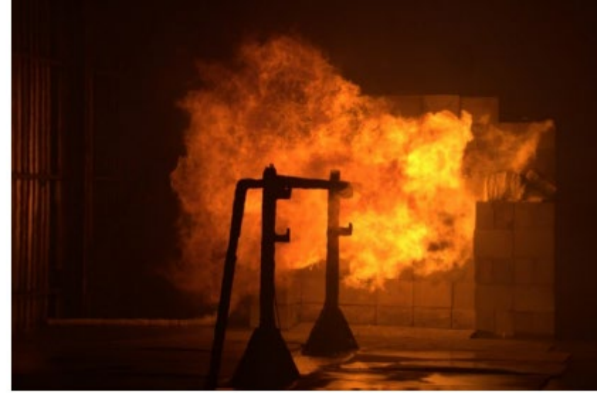
Figure 3 ISO22899-1 jet fire test
